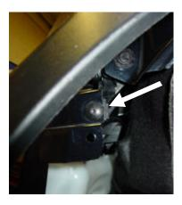
With the wheel arch trim loose at the front it is possible to access and remove the T25 Torx screw that secures the front panel.
