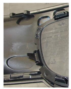
Prior to removing the lower grill, the ambient temperature sensor is removed from its retaining slot in the grill. The sensor is moved to the rear of the side / fog light and secured with the supplied tie wrap.
