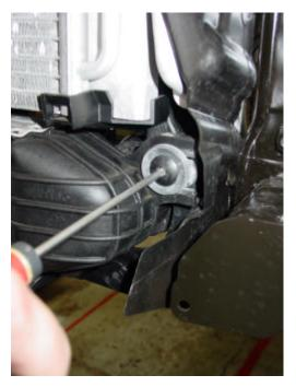
The Original intercooler mounting screws (T25 Torx) can now be removed from each side of the intercooler.
