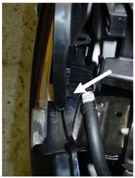
In order to release the lower edge of the grill it is first necessary to remove the lower chrome cover. At each side there is a plastic tab that requires raising slightly to release the clip that secures the chrome strip.
