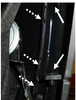
With the fasteners removed the wheel arch liner can be pulled away. The outer wheel arch trim is secured by two of the pushpin type fasteners that require removal and three plastic tabs (dotted arrow) These can be "released" by pushing with a flat blade screw driver.
