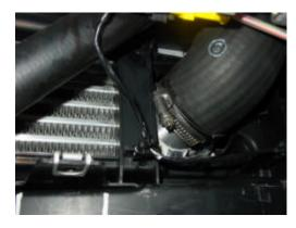
The Original intercooler can now be removed. It may be easier, when stood at the front of the vehicle to remove your right hand side first before removing your left hand side.
