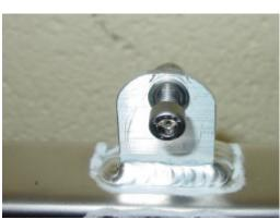
In the centre at the top of the new intercooler there is a bracket that will secure the intercooler to the metal crash bumper. In order to attach this, a 6.5 mm or ¼" hole requires drilling. To facilitate this, with the intercooler in place, mark the required position of the hole on the crash bumper. Now remove the intercooler. It is strongly advised that in order to drill the crash bumper it is removed from the vehicle first, to prevent any damage to the air condenser radiator.
